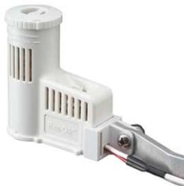
This sensor type device connects to an existing irrigation controller, either wired or wireless, and acts to block the controller from running irrigation when a preset volume of rain is received. This low cost apparatus is easy to install especially when using the wireless model. The sensor can be installed where it will have the best opportunity to catch rainfall and the receiver unit is installed next to the controller to which it is wired.
