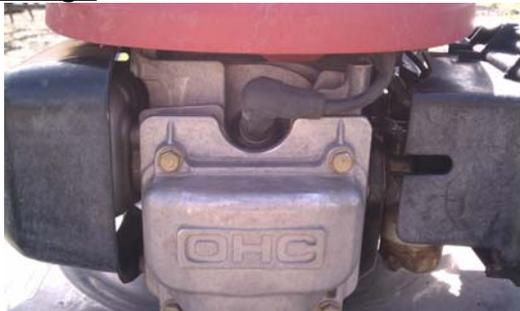
Many people never even think of changing the spark plugs if the machine is working properly. The truth is, spark plugs wear out over time under normal operating conditions. Changing the spark plug can bring a mower back to life and eliminate countless extra pulls to start the machine. Even if a mower is
