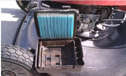
Something often overlooked is a clogged air filter. A clogged filter can reduce the power of a mower and also lower its fuel economy. With heavy equipment use, two filter changes a year will make a significant difference over the lifetime of the machine.
