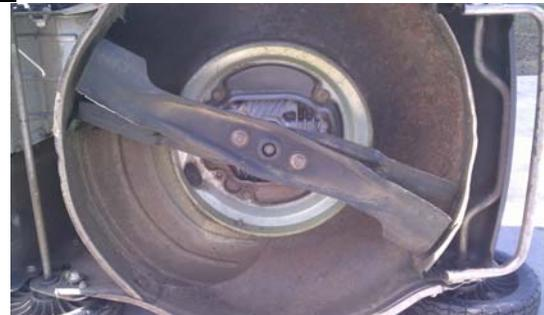
Sharp blades are one of the most important aspects of a mower. A sharp blade cuts the grass evenly and with minimal effort. A dull blade actually rips the grass and can cause an uneven cut. To insure the mower provides the best cut, change the blades or have the blades sharpened at a local lawnmower service shop every other month.
