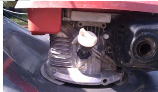
Oil is the blood of your mower; mowers need to have their oil changed throughout the year to remove particulate contamination caused by wear and tear. The frequency of oil changes is dependant on how often and how long the mower runs. The longer and harder the machine is worked, the more frequent the oil will need to be changed. For home use, an oil change in the spring and fall should be plenty to keep things properly lubricated.
